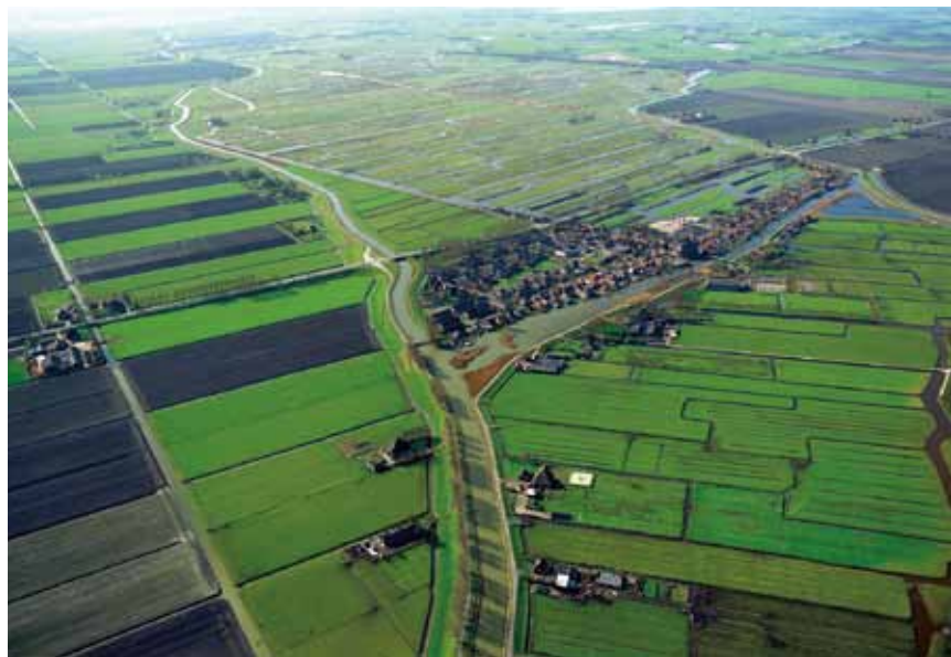
Polders. On the left is the Beemster, drained in 1612, and above right the Schermer, drained in 1635. Both have a ring dyke and a ring canal. Between the two polders is a strip of older peat meadow where the village of Schermerhorn is located.
