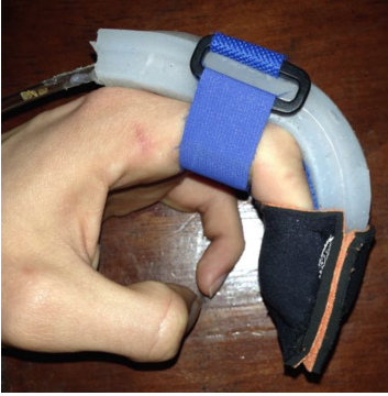
Fig. 34. A one finger prototype was made to resist motion of the finger in bending [44].
