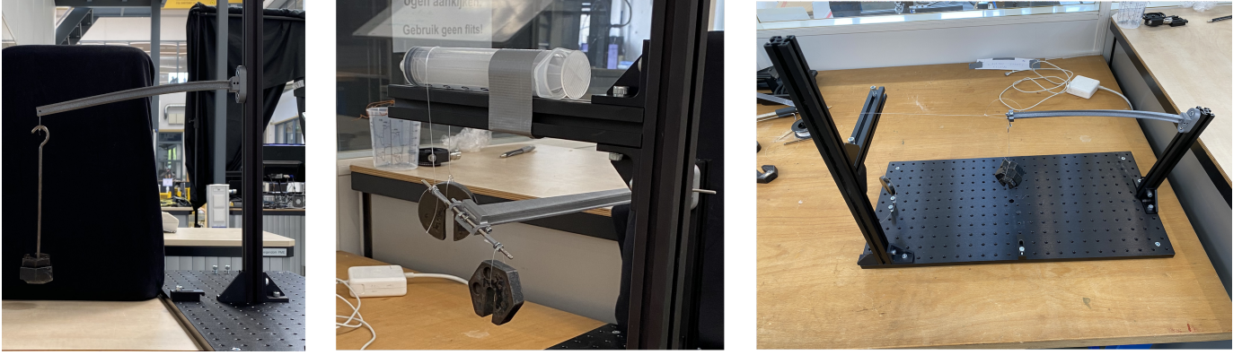
Figure 7: The critical load is validated by attaching weight at the free end of the cantilever (left). A pure moment is applied to the free end of the beam to determine the resulting angle in a state without preload by placing a moment arm to the centre of the cross-section of the beam and applying equal but opposite loads on each end of the moment arm (middle). The preload is applied at the free end of the beam by a horizontal component by a weight hung around a pulley and a by vertical component by a weight attached directly. The moment about the longitudinal axis is applied by placing the weight, representing the vertical component of the preload, on a small moment arm at a slight distance from the centroid of the cross-section
