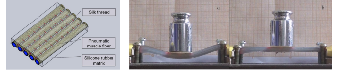
Fig. 25. The pneumatic fibres are embedded in soft matrix material to form a variable stiffness composite (left). A prototype is loaded in bending for both the soft (right, a) and stiff state (right, b) [34].
