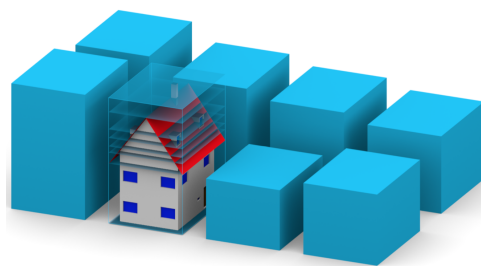
Figure 3: Seven different LOD1 block representations for the same building (in LOD3) when different height references are used. Source: (Biljecki et al., 2014).
