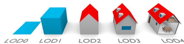
Figure 2: The five LODs as specified by the OGC for CityGML 2.0. Source: (Biljecki et al., 2016).
