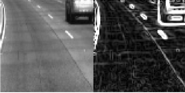
Figure 2: Input 80x80 image before and after Sobel edge filter
