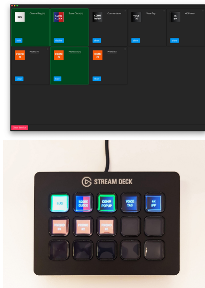
Figure 6: Trigger launcher (top) and hardware device StreamDeck (bottom) for operating it more conveniently
