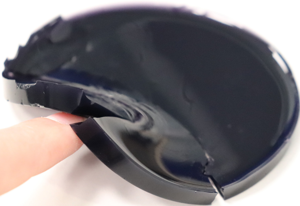
Figure 8.1 - Cracking behaviour of MAR medium
