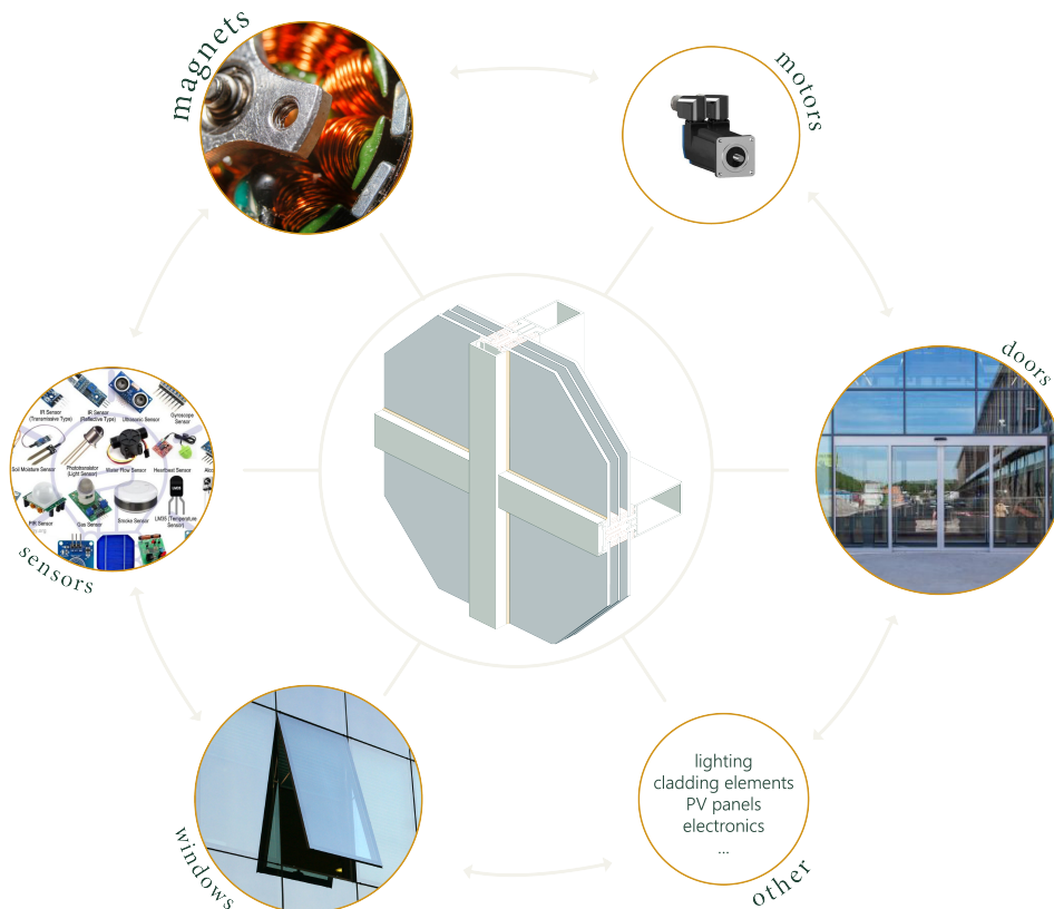
Figure 2.11: Elements of a curtain wall façade
