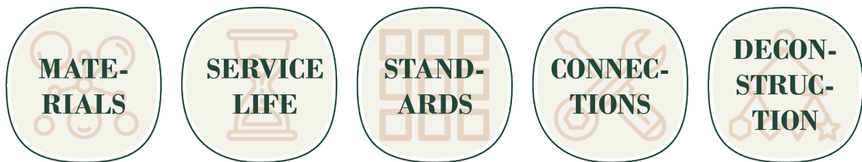
Figure 2.8: 5 principles to consider for DfD according to GXN [Merrild, 2016]
