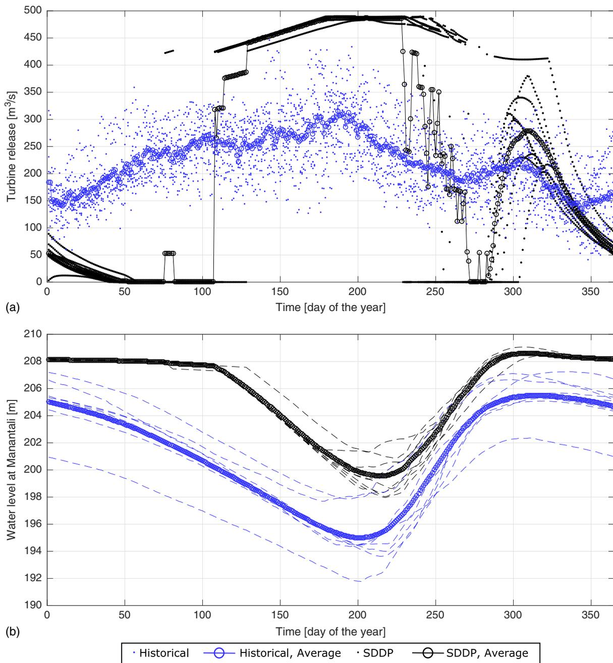
**Fig. 4.** (a) Turbine release; and (b) water level at Manantali. Solid lines show results from SDDP maximizing energy production.
