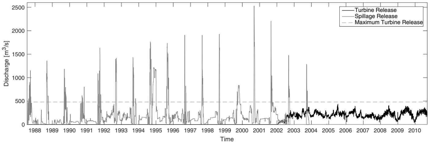
Fig. 1. Historical operation of Manantali, 1988–2011: observed turbine releases (solid line) and spillage release (gray line).
