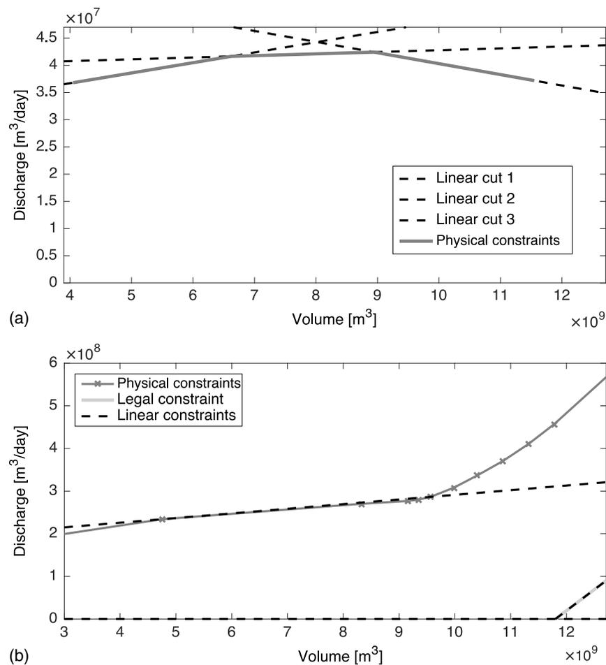
**Fig. 3.** Constraints depending on the reservoir volume. Continuous lines show physical and legal constraints and dashed lines indicate linear cuts included in the optimization: (a) maximum turbine release; and (b) maximum spillage release.
