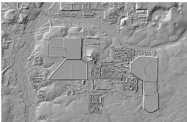
Fig. 3 The amplified scale of the transformed landscape through phosphate mining, Florida. A clay settling pond, a 10 m high dam can reach dimensions of 2 km by 2 km, creating almost arena-like sceneries.
