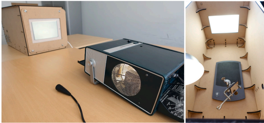
Fig. D2. Replica of Hess's pupil apparatus. The top lid of the box was closed during the measurements.
