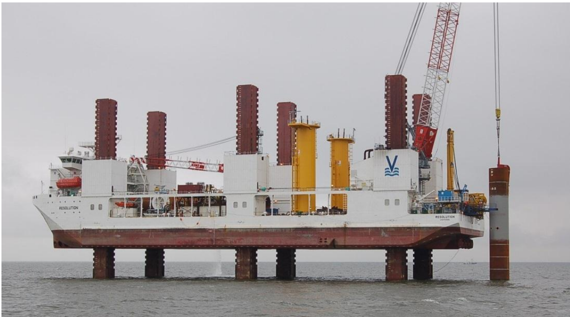
Figure 18.2 – jack-up vessel with hollow pile legs [www.windmanagement.co.uk]
