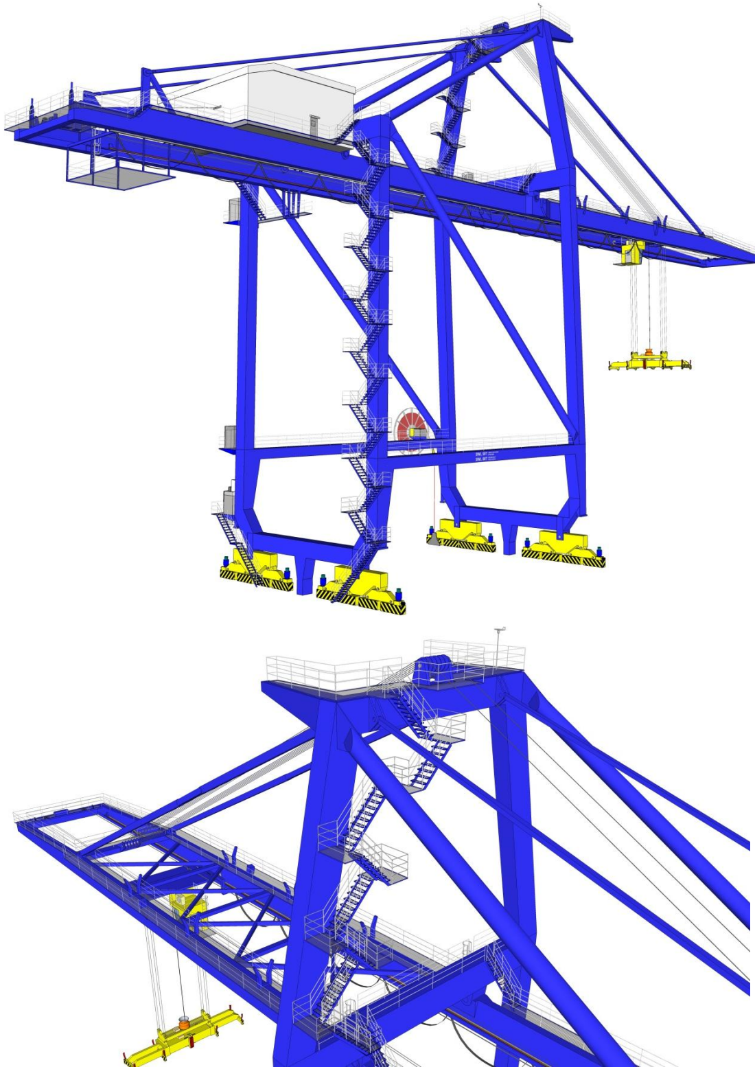
Figure P.1 – impression of highly detailed scale model of a post panamax STS crane, used to determine the governing wind surface and wind load.
