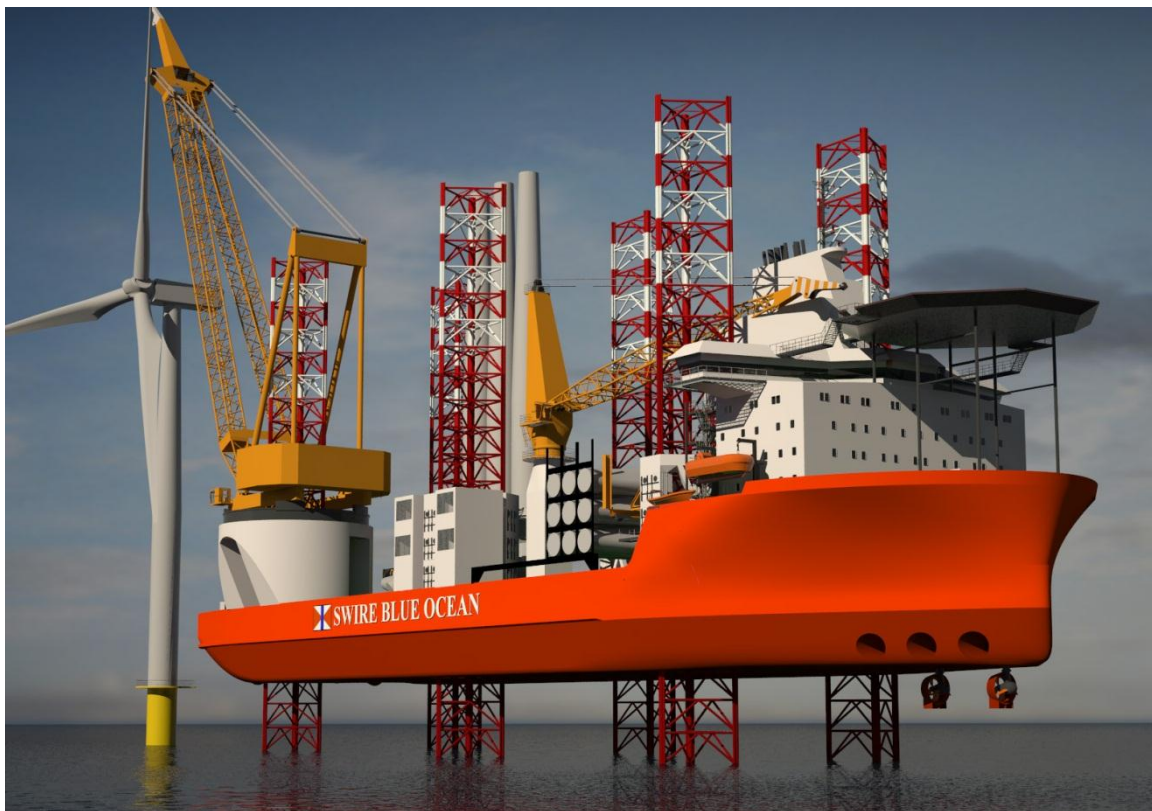
Figure 18.3 – jack-up vessel with framework legs [www.knudehansen.com]
