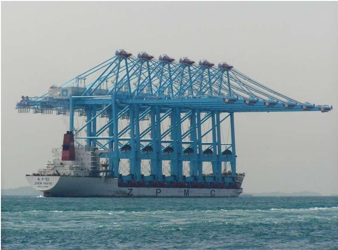
Figure 18.1 – transportation method of ship-to-shore cranes [www.cochinsquare.com]
