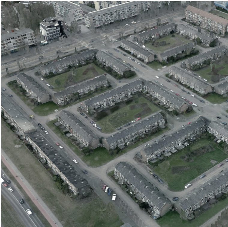
Fig. 30. Repeating L-shape arrangement of housing blocks enclosing courtyards in Roland Holsbuurt (" Amsterdam · Netherlands ", 2023)
