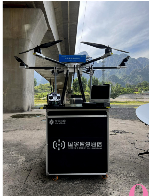
Fig. 3.13, Communication Base Station Drone-based emergency communication aerial base station Image source: http://v.china.com.cn/zhuanti/2023-08/03/content_98140444.htm
