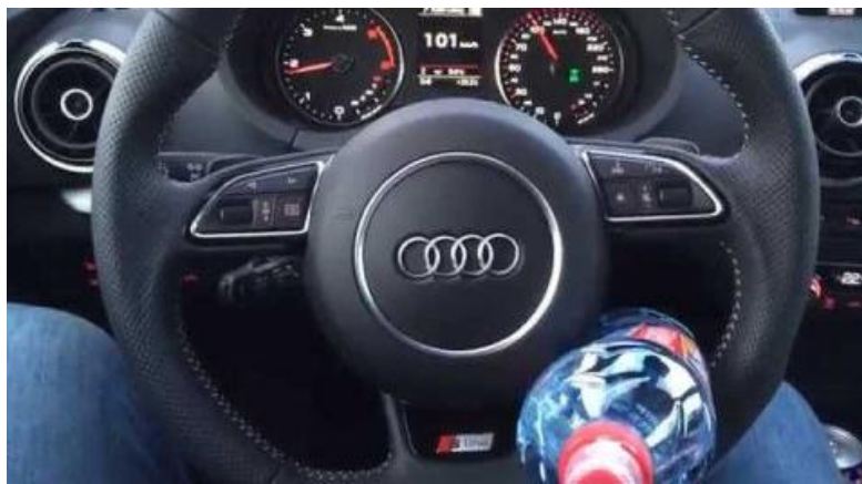
Figure 2: Placing a bottle on the steering wheel to circumvent the hands-free warning. Source: Adopted from https://www.youtube.com/watch?v=qi2oIRMwmZY
