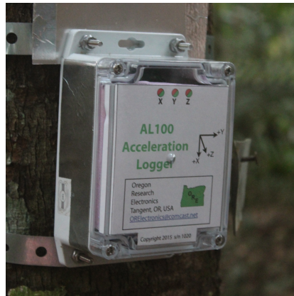
Figure 1. Picture of an accelerometer installed on a tree.
