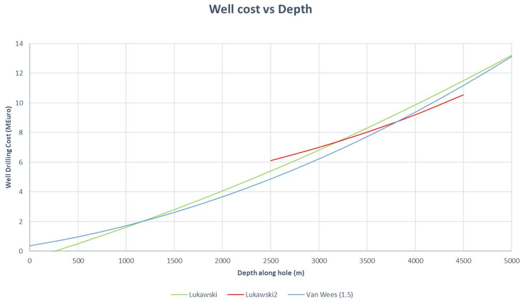
Figure 8: Well cost as function of Depth. Equation 1 is taken from van Wees(x), where x represents the well cost scaling factor. Equation 2 and 3 are referred to as Lukawski1 and Lukawski2.
