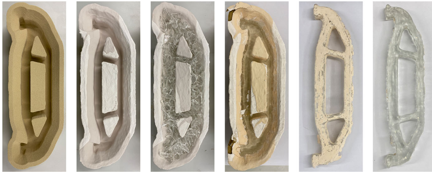
Fig. 11 Geometry 4, sample CCSX2F4b. From sand mould to glass piece. Same steps as in Fig. 10
