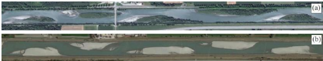
Figure 1. Two rivers with similar hydrogeomorphological parameters and different conditions for the alternate bars. (a) Fully vegetated bars on Isere river, near Arbin France. (b) Bare bars on Alpine Rhine, near Meierhof, Liechtenstein.
