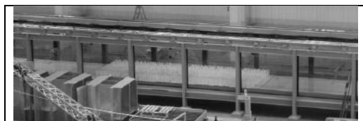
Figure 1. Sideview of the 6 m long array of rigid cylinders at the center of the 18 m long sand bed.
