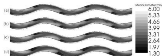
Figure 2. Mean surface grain size, for the channel with crossing angle \omega = 20^\circ . (a) - (c) are from the unsteady flow run ((a) Q_w = 0.026 m 3 /s, (b) Q_w = 0.07 m 3 /s, (c) Q_w = 0.13 m 3 /s) and (d) is from the constant-discharge run ( Q_w = 0.07 m 3 /s).
