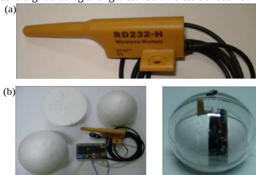
Figure 1. Dynamic scouring observation technologies (a) Long-distance wireless transceiver (RD232-H); (b) wireless tracking device
