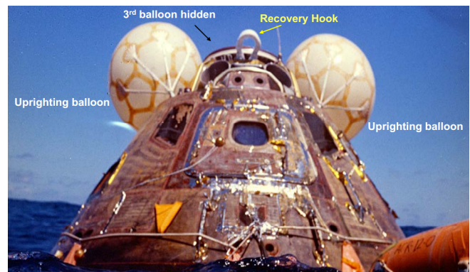
Figure 4.17: Up-righting balloon with hook [35]
