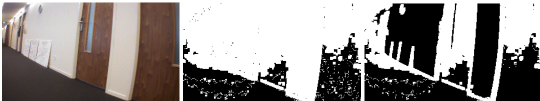
Figure D-11: Comparison different thresholds RGB color matching. Left to right: front camera image, thresholds: R \leq 2, G \leq 2, B \leq 2 , thresholds: R \leq 2, G \leq 2, B \leq 1.999
