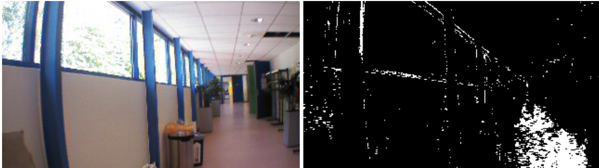
Figure D-6: Left to right: front image, HSV averages threshold segmentation with thresholds H \leq 0.5 S \leq 0.1 V \leq 0.1
