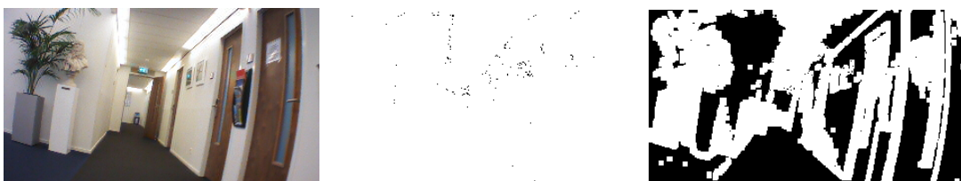
Figure D-10: Comparison different thresholds RGB color matching. Left to right: front camera image, thresholds: R \leq 2, G \leq 2, B \leq 2 , thresholds: R \leq 2, G \leq 2, B \leq 1.999
