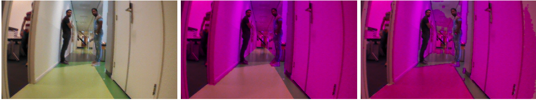
Figure D-24: Left to right: Front image, segmentation by hand-labelled image, segmentation by Laws' mask, pink represents obstacle
