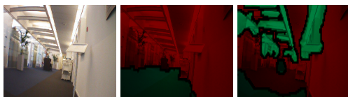
Figure 15: Example segmentation, all pixels classified as obstacle are made red, non-obstacle are green. Left to right: input image, hand-labelled image, Ulrich
