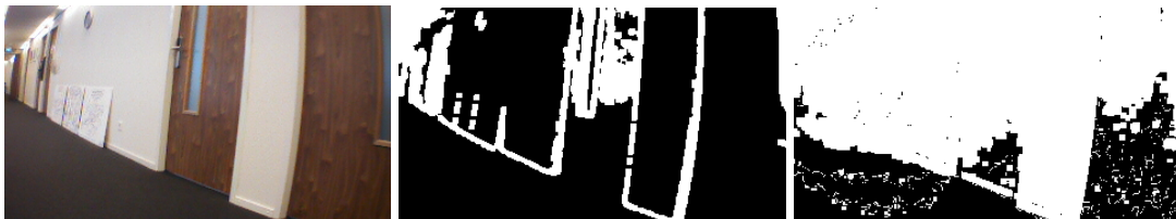
Figure D-9: Comparison different thresholds RGB color matching. Left to right: front camera image, thresholds: R \leq 1.97, G \leq 1.97, B \leq 1.97 , thresholds: R \leq 2, G \leq 2, B \leq 2
