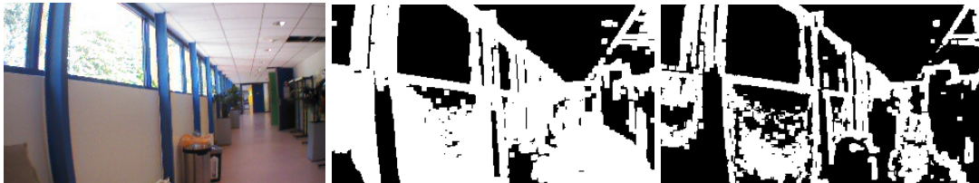
Figure D-12: Comparison different thresholds RGB color matching. Left to right: front image, threshold values: R \leq 1.97, G \leq 1.97, B \leq 1.97 , threshold values R \leq 1.89, G \leq 1.88, B \leq 1.70
