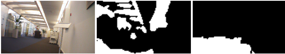
Figure E-7: Example segmentation on dataset 1. Left to right: input image, Ulrich thresholds based on dataset 1, ground truth
