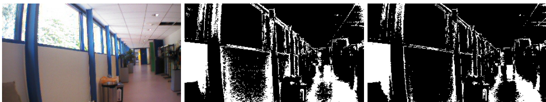
Figure D-4: Comparison different thresholds RGB color matching. Left to right: front image, threshold values: R < 40 & G < 65 & B < 55 , threshold values R < 32 & G < 40 & B < 60
