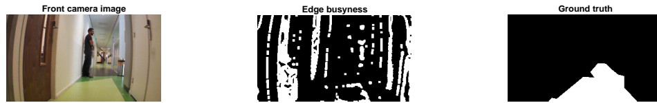
Figure D-18: Example of a bad segmentation when using the edgeness feature. Left to right: input image, resulting segmentation, ground truth
