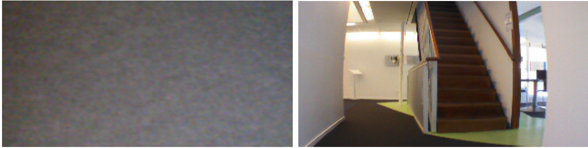
Figure C-3: Example of bottom camera image with matching front camera image. Bottom image: gray uniform floor, front image: black and green floor
