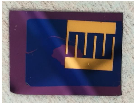
Figure 2.2. CVD graphene on top of SiO 2 with electrodes
