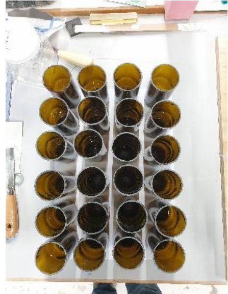
Figure 53 – Top view of the cut Bottles after sanding
