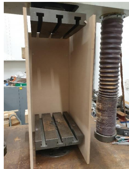
Figure 54 – Safety casing made from MDF surround the pressure plates
