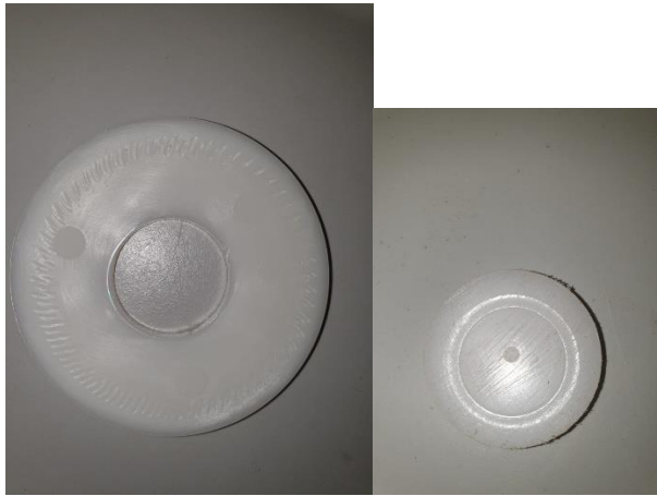
Figure XX - Pictures of the deformed plastic elements (left: M20 Nylon ring, right: POM disk)
