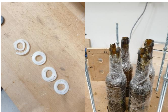
Figure 56 and 57 – Torn nylon rings after failed test. Picture showing crushed finishes of the bottle, indicating a fault in the test procedure.
