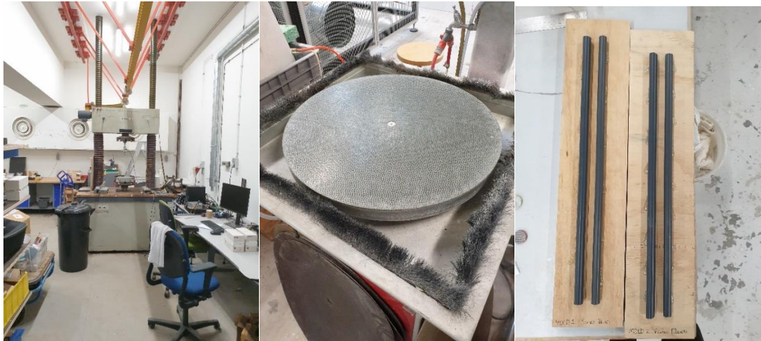
Figures 49, 50 and 51 – The allocated lab room with machine, sanding machine for the cut-bottles, molds for gluing the samples
