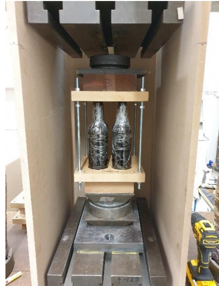
Figure 55 – Whole-Up configuration set-up before testing
