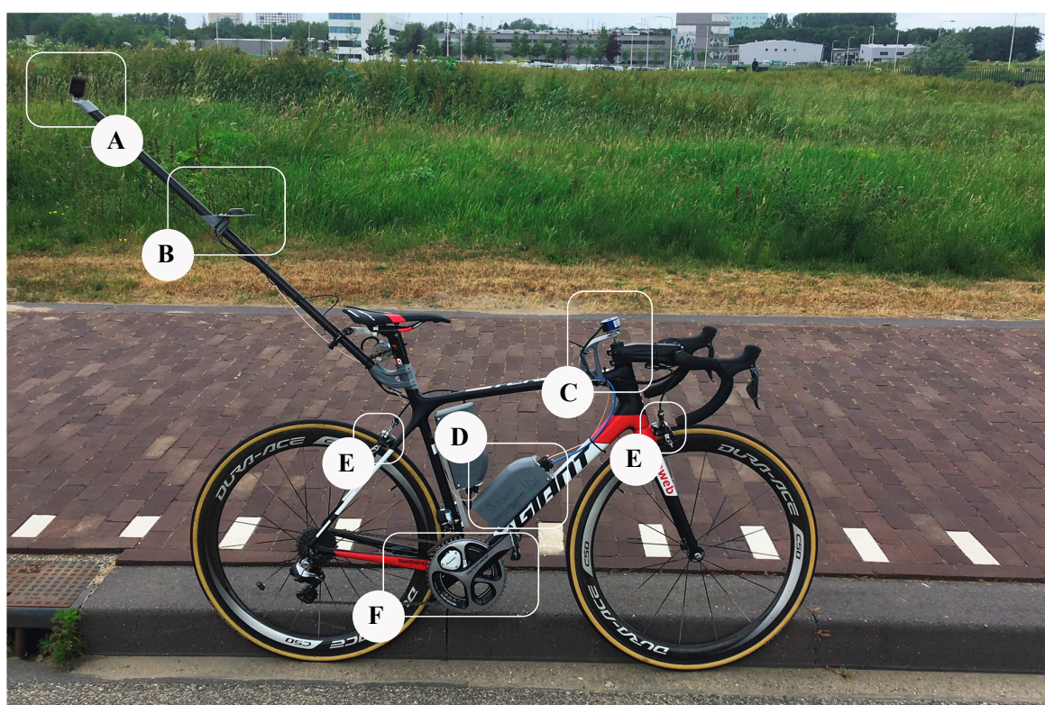
Figure 1. Measurement system installed on a bicycle. (A) GoPro camera and mount to record rider posture; (B) GNSS antenna to measure rider's position on the road; (C) optical encoder to measure steering angle; (D) IMU to measure roll angle and data acquisition system; (E) strain gauges on brake shoe to measure brake force; (F) velocity sensor and power meter.
