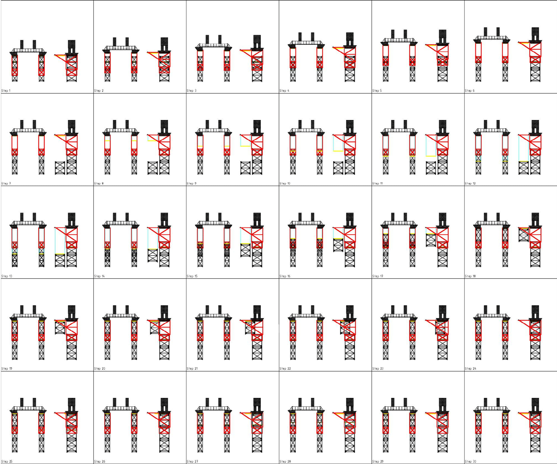
Figure C-66 Climbing frame top building sequence
