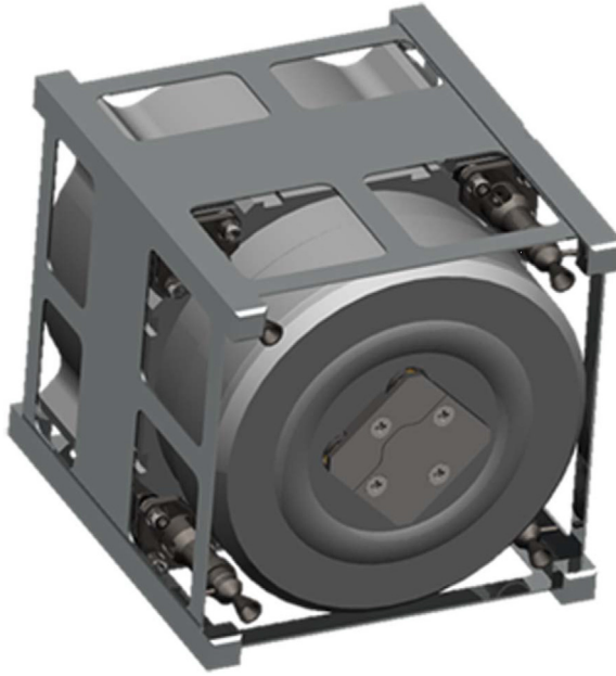
Figure 18.6 The MPS-120 modular propulsion system from Aerojet Rocketdyne [7].
