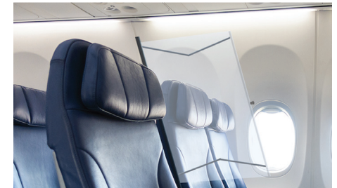
Vision Systems developed a lightweight transparent barrier to separate passengers.
