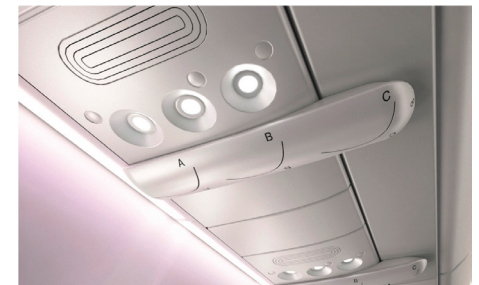
AirShield by Teague uses a 3D-printed module to create "air blades" which control droplet spread more effectively.
