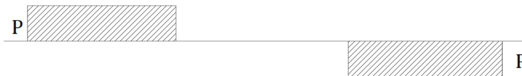
Figure 107 Shear force diagram for prismatic beam shown in Figure 105
