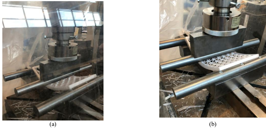
Fig. 10a) Honeycomb recycled PET core at a deflection of 50 mm, b) Truss recycled PET core at a deflection of 50 mm.
