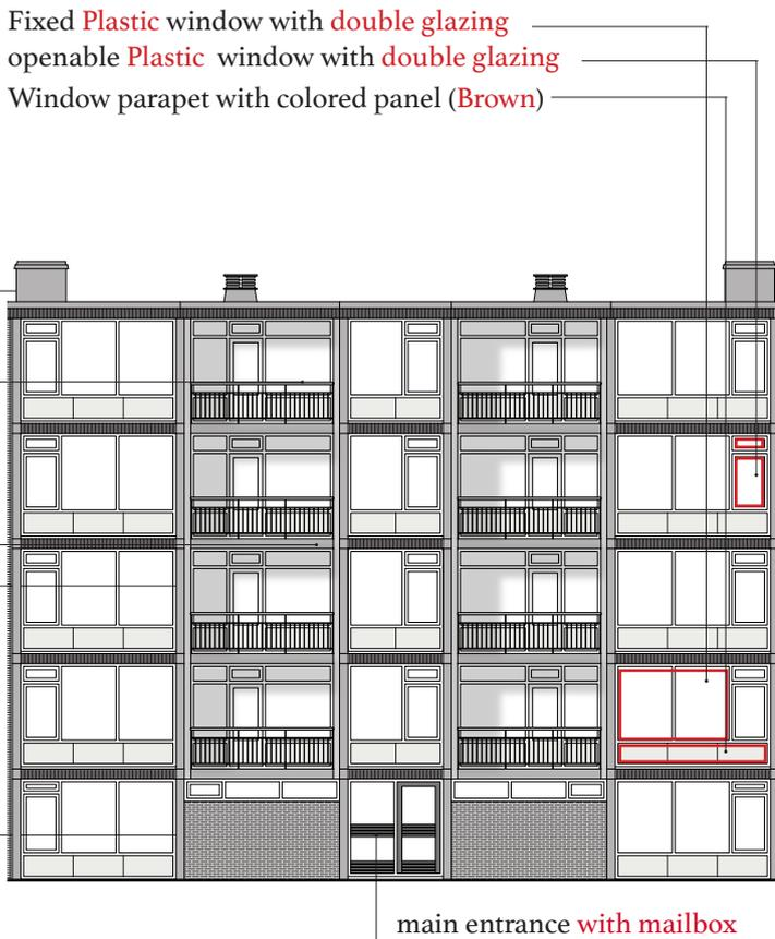
Figure 1.3.26. Front elevation (After renovation) 1:200
