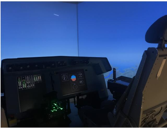
**Fig. 5 Fixed-base simulator in aircraft configuration**
