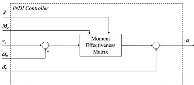
Fig. 2 Schematic block diagram of the INDI controller
