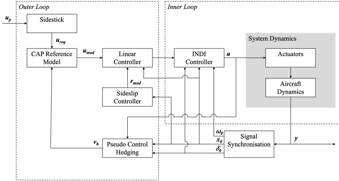
Fig. 1 Schematic block diagram of the controller structure
