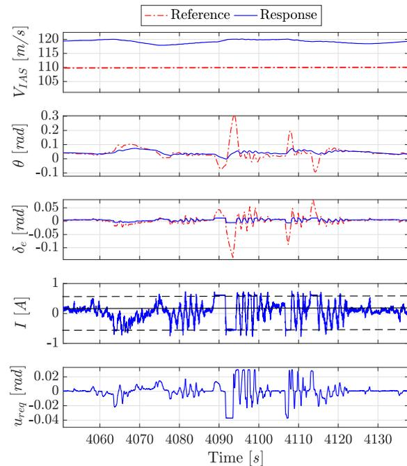
**Fig. 17** Longitudinal tracking response ( $V_{ias} = 120$  [m/s] FL130)
