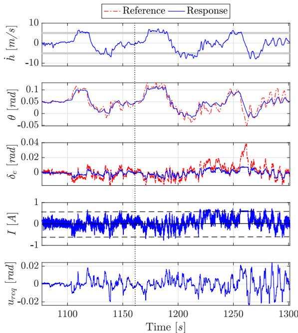
**Fig. 16** Longitudinal tracking response ( $V_{ias} = 110$  [m/s] FL130)
