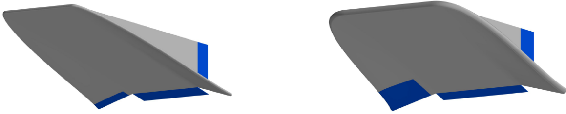
Fig. 19 Predicted shapes for optimal cross-range (left) and heat load (right).
