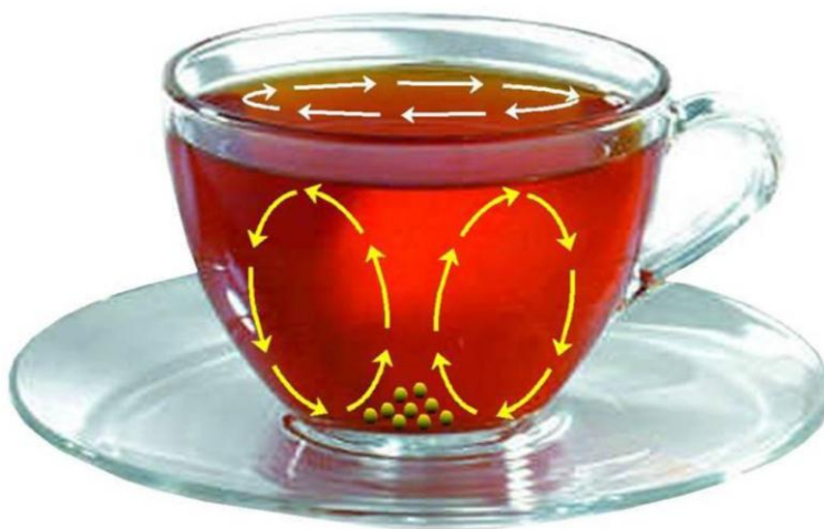
Fig. 9-6: Particle motion due to hydrostatic pressure differences (Mosselman 2010)
