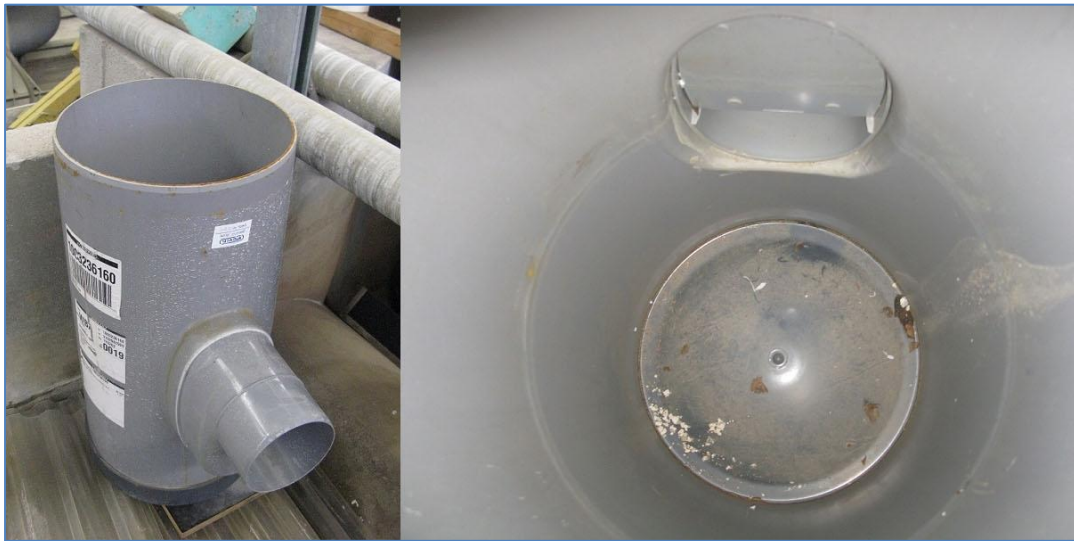
Figure 30 - The original gully pot
