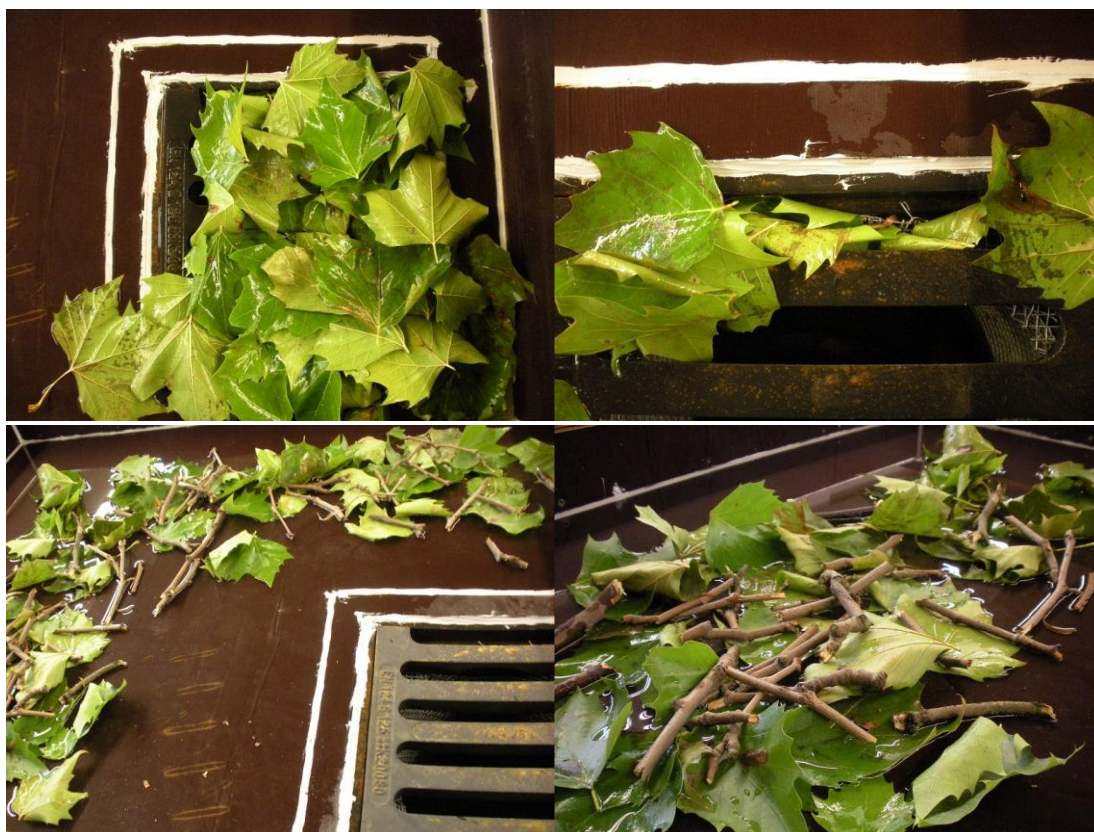
Figure 46 - Testing with real fresh leaves and braches
