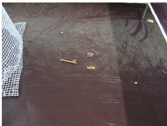
Figure 64 - Samples remained in the gully pot for testing alternative 4
