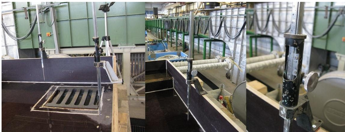
Figure 40 - The device to measure the water level on the test table
