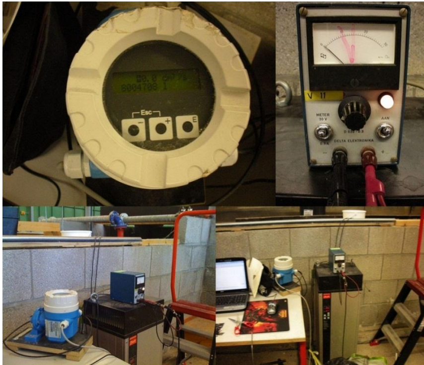
Figure 39 - The device to control and read the flow capacity
