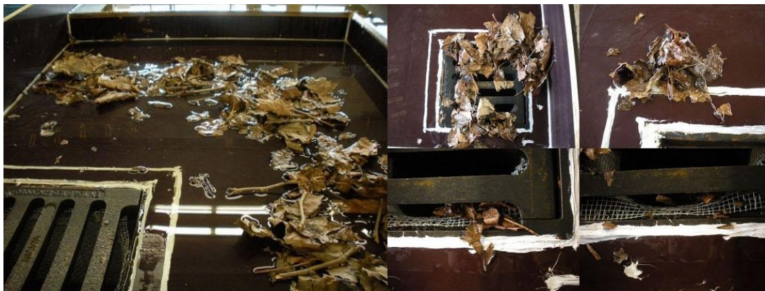
Figure 45 - Testing with dry leaves and branches
