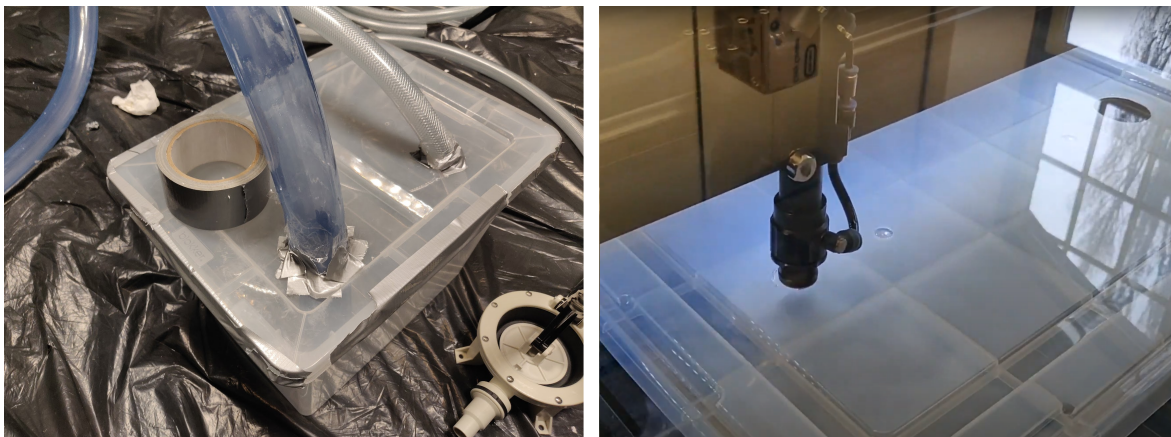
FIGURE 3.15: With the small buffer of 20 litres an attempt was made to stop the leakage by applying duct tape around the lid and where the pipe goes through the lid (left). Fortunately, there was the option to use a laser cutter. The holes were laser drilled in the diameter of the pipes (right).
