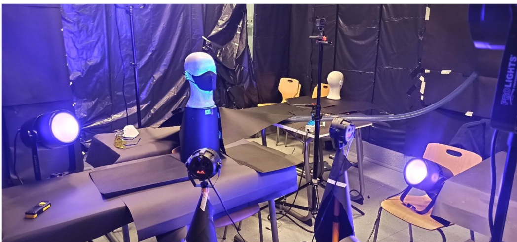
FIGURE 2.16: Setup of the manikin with a face mask. A long PVC tube is connected from outside the experiment site with the box. The manikin is resting on top of the box (Ortiz, Ghasemieshkaftaki, and Bluysen, 2021). Used with permission from the author.
