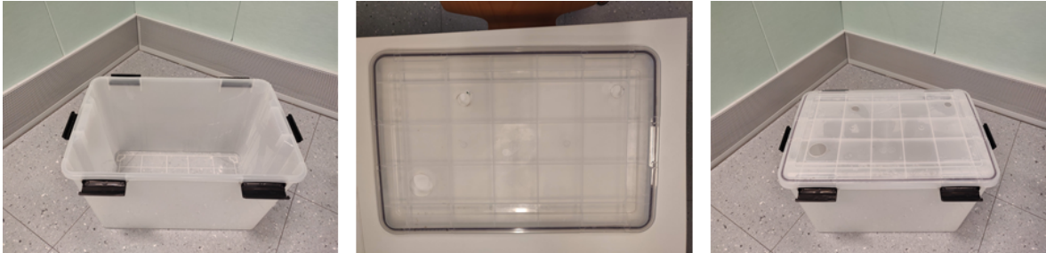
FIGURE 3.21: A 70-litre buffer with an airtight lid. There are three holes in the lid. The pipes can be inserted through these holes.
