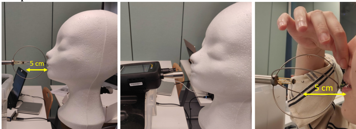
Manikin with the air velocity (left) and particle counter (middle). Human subject breathing through her mouth (right).
