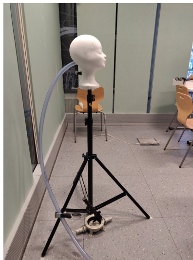
FIGURE 3.8: Unfinished setup with only the manikin on the tripod. The pump was connected with the tube during the baseline measurements. The indoor air of the room was used as the medium, instead of glycol.
