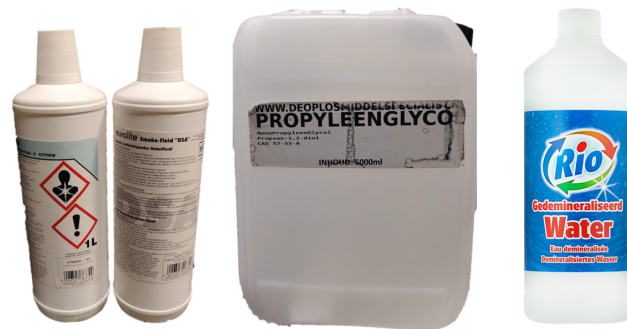
FIGURE 3.12: Different types of glycol concentrations were used. The viscosity of glycol is high and can be diluted by the demineralised water, making it easier for the machine to convert the liquid into the fog.
