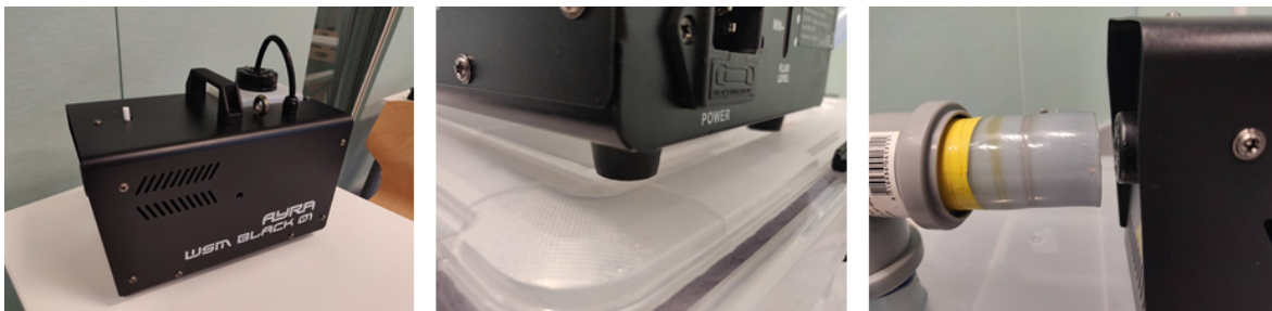
FIGURE 3.25: The container of the fog machine is filled with glycol and demineralised water. A ratio of 9:1 was used. The fog machine was placed on top of the lid and the legs fit exactly in the cavity. A small open distance between the pipe inlet and the nozzle is necessary. Otherwise, no fog will enter the buffer.
