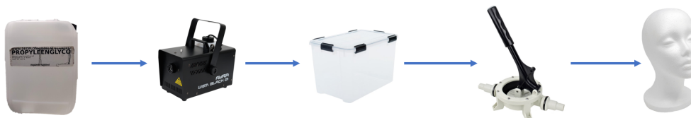
FIGURE 3.11: The medium is poured into a small container of the fog machine. The fog machine is turned on and fog comes out of the nozzle. A pipe is placed in front of the nozzle, which is connected to the buffer. The fog is collected in it. When enough fog is accumulated, it is transported to the manikin through the pumping mechanism. The manikin exhales the fog.
