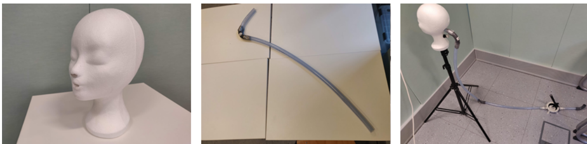
FIGURE 3.26: The final step is to assemble the manikin on the tripod. The cavity within the manikin was carved out with a screwdriver. The pipe was connected with PVC elbow tubes and inserted in the back of the manikin. The pump is connected to the other end of the pipe.
