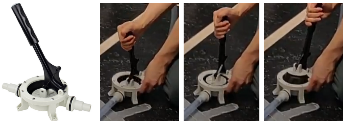
FIGURE 3.17: The Nuova Rade Handlenspomp (left). The pumping mechanism is displayed with the three figures. In this example, the inhaling process is demonstrated as the handle is pulled back. Simultaneously, the other hand must press the pump to the ground. Otherwise, it will shift during the process (right).
