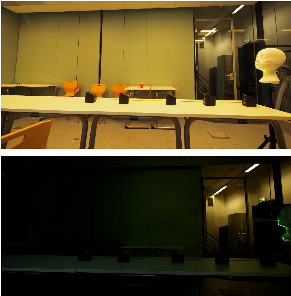
FIGURE 3.28: Overview of the setup to capture the airflow pattern by placing the camera next to it to create a side view (top). During the experiment, the fog was not visible enough (bottom).
