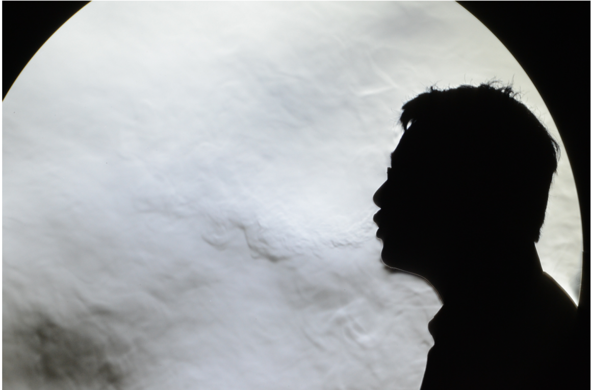
FIGURE 2.11: The subject stands one meter in front of the spherical mirror and exhales. The visual of the breath can be seen due to the difference in temperature of the breath and room (Tang et al., 2011a). Used with permission from the author.
