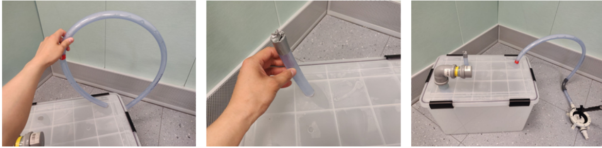
FIGURE 3.24: A pipe with a diameter of 25 mm is inserted at the other corner of the lid. This is to transfer the fog from the buffer through the pump. Another pipe is inserted and the other side is covered with duct tape.
