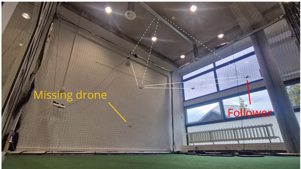
Figure 4.9: RAL Experiment with 5-drone formation at t = 45 after missing a drone
