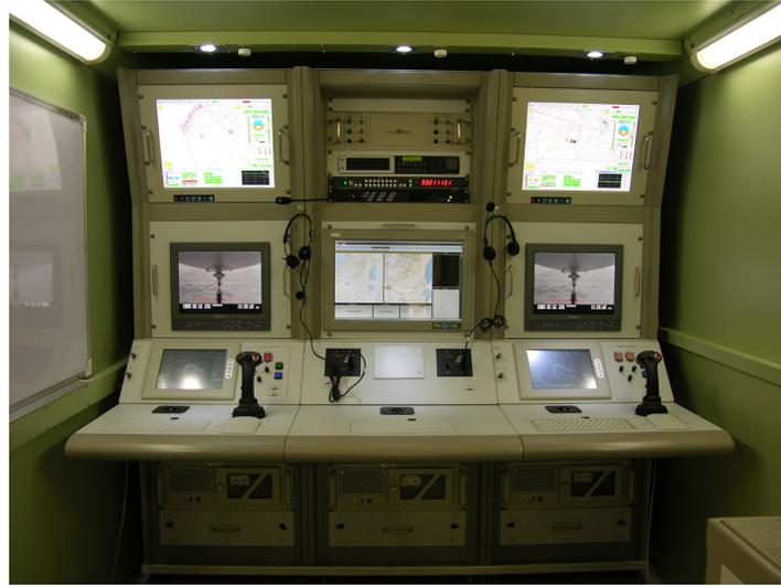
**Figure 1-3:** An example ground control station (GCS) used to teleoperate UAVs. Pilots receive only visual feedback of the UAV states. The GCS pictured is manufactured by Aeronautics Ltd.(Aeronautics, 2007).
