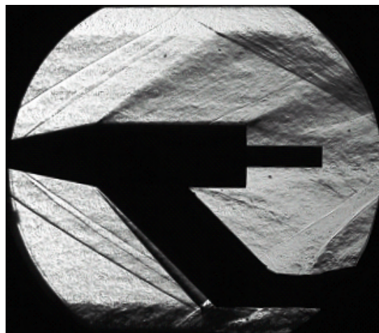
Figure 5.7: Instantaneous Schlieren snapshots for L/D = 1.2 at M_{\infty} = 2.2, p_0 = 2.5 \text{ bar} , without exhaust plume
