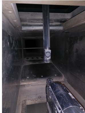
Figure 4.18: Laser probe inside the wind tunnel
