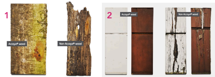
1) 15 year canal lining test 2) 10 year external coating test
