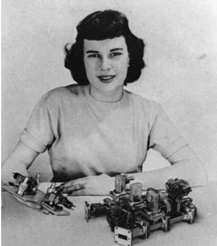
Figure 1.1: Comparison of a tri-plate with a waveguide-based circuit. [1]
