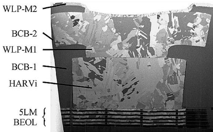
Figure 2.7: Cross section of an inductor fabricated using Cu electroplating and BCB film separation [21]. 5LM BEOL refers to 5 layers of metallization at the end of a CMOS process. Inductor is fabricated using WLP-M1 layer and BCB-1 is used for separation.
