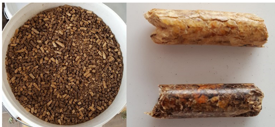
Fig. 1. Wood pellets used in the experiments; a bucket of mixed pellets (left), the two different types of wood pellets in a close-up (right).
