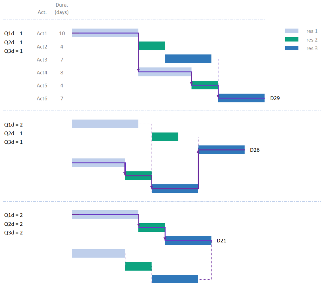
Figure 6.3: Gantt chart of a part of case 2 schedule, with different numbers of teams ( Q_{rd} ).
