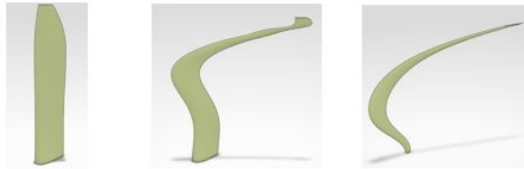
Fig. 3.5 Two optimized blade geometries and the reference blade from the optimization study of Hu. [13]
