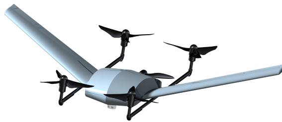
Figure 23.1: Final design of the silent delivery drone.
