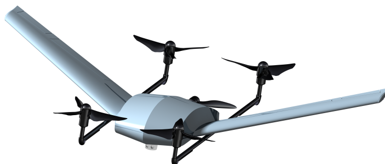
Figure 2: Overall configuration of the silent delivery drone
