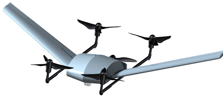
Figure 15.1: Overall configuration of the silent delivery drone
