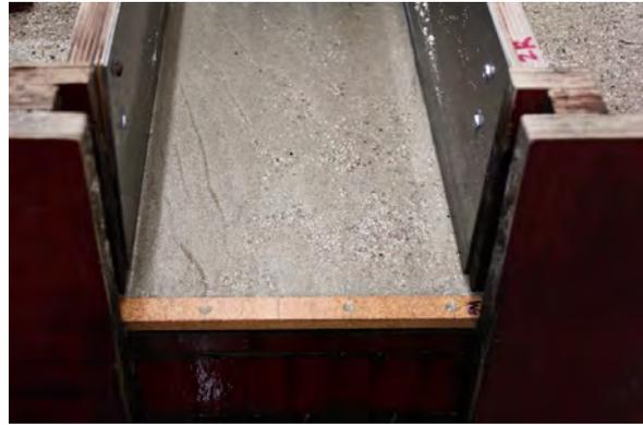
(b) Downstream installed weir
