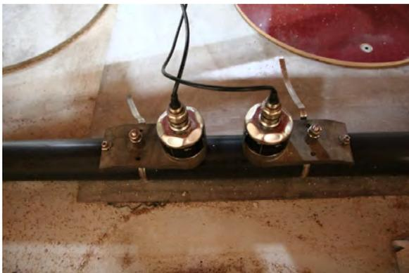
(a) Two sensors connected to pipe
