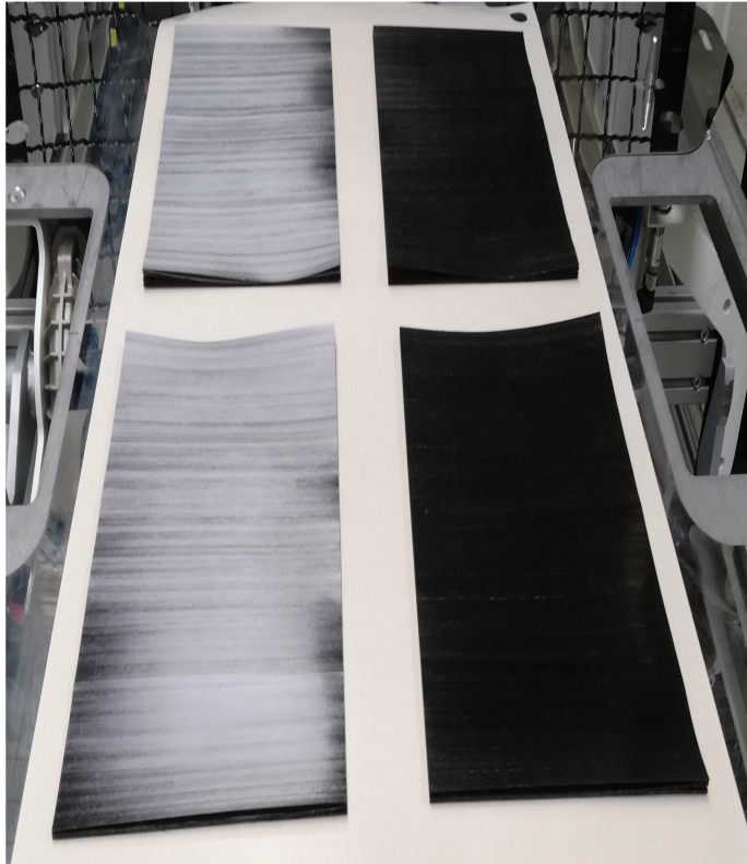
Figure 4.17: Laminate Configuration before the press
