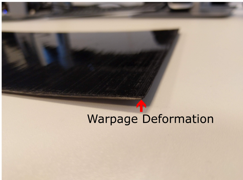
Figure 1.3: Warped laminate from Falcon Line
