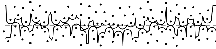
Figure 4.1: Fiber distribution obtained with the algorithm by Melro et al. [52] along with matrix interlayer (vertical distance between solid lines), deduced with central interface line (dashed line).
