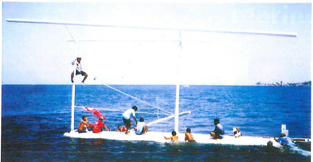
Caught in an off-moment, one of the rapid fleet of Sandeq ('pointed') boats raced by the merchants and fishermen of Sulawesi, a small island north of Java. These triple-hulled craft range in length from 5m to 15m and have regularly been recorded at speeds in excess of 25kt. A huge lateen rig powers the Sandeq, for which a 200-mile, four-stage inter-island offshore contest is the highlight of the annual race season
