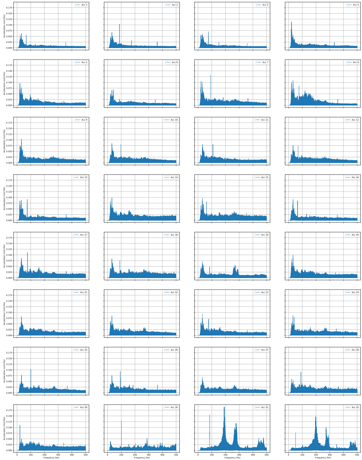
Figure A.3: Fourier transform of all sensors recorded on the 11th of October 5:14 AM with a high-pass filter of 20 Hz.
