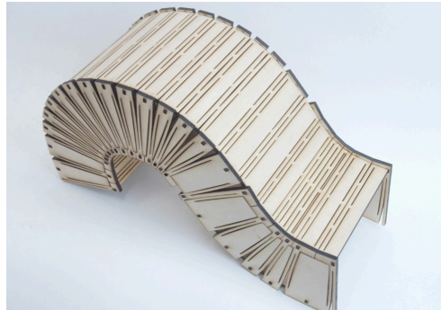
Figure 8 Final shape of designed piece. Flat sides are constructed using deformation A and curved surfaces are constructed using deformation B.
