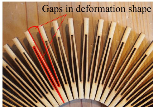
Figure 5 Heterogeneous pattern A. There are smaller gaps in pattern than in the homogeneous pattern in Figure 4.
