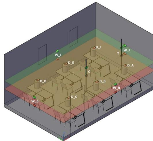
Note: measurement locations at 1.1m were marked in red and at 1.6m were marked in green.
